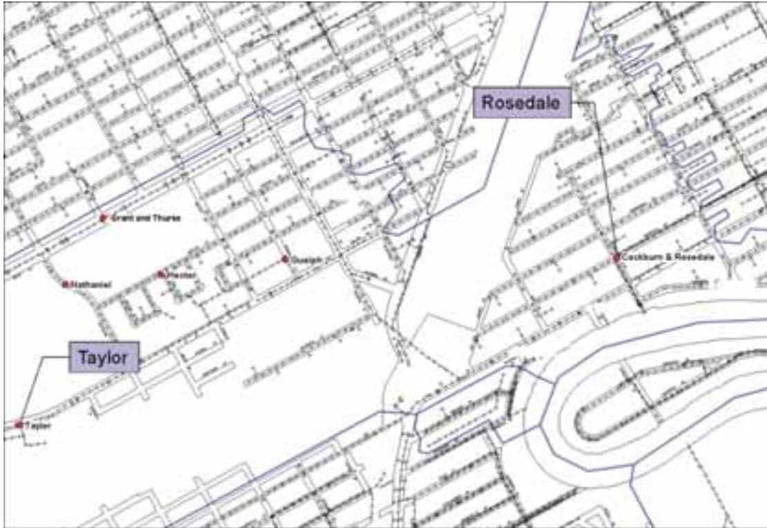
Figure 3-15 – 2006 Collection System Flow Monitoring Locations
