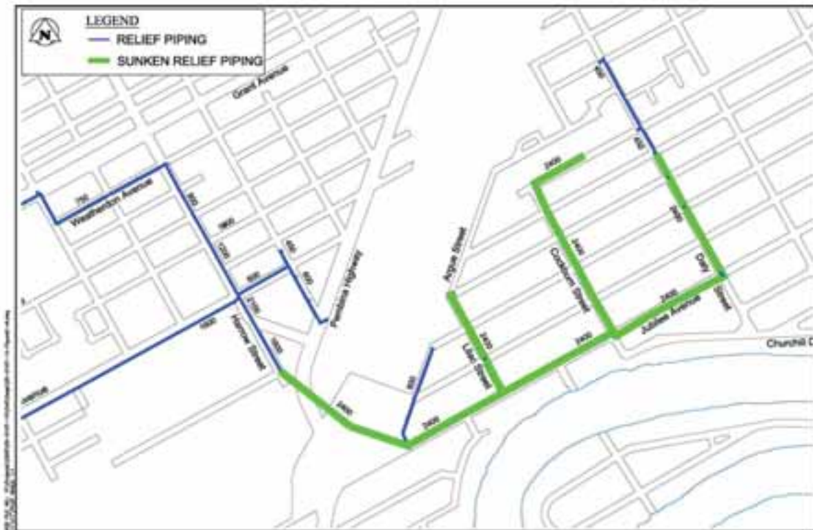
Figure 12-13: Modified Relief Piping – Sunken Relief
