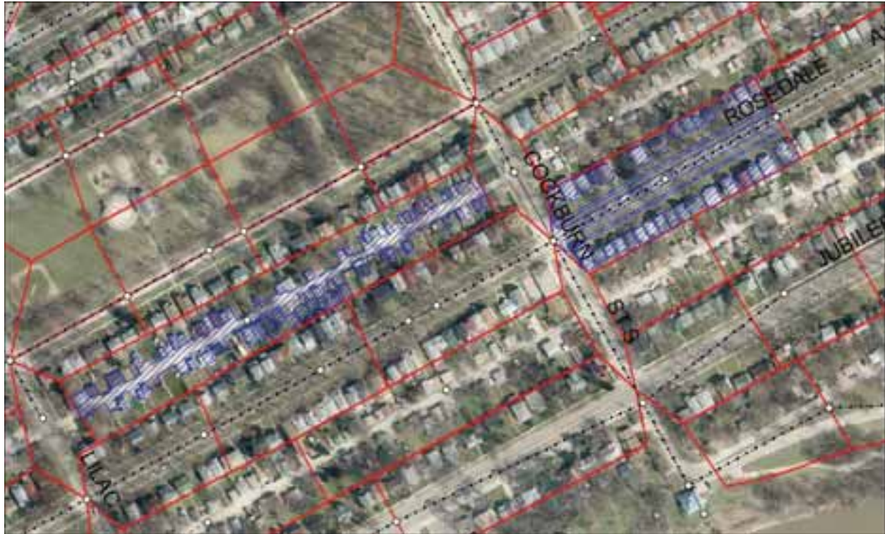
Figure 2-3: Sample Calculations of Percent Imperviousness for Residential Area
